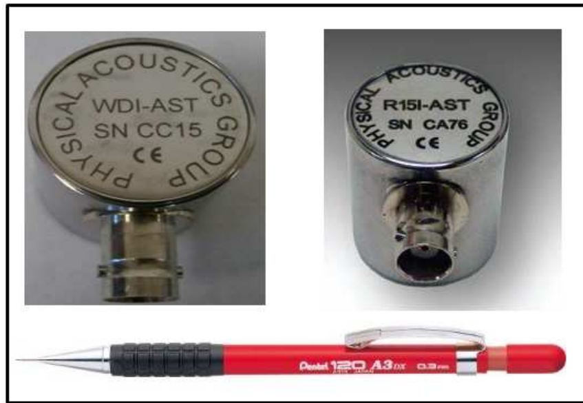
Figure 3.2. AE sensors and 0.3 mm lead pencil.
